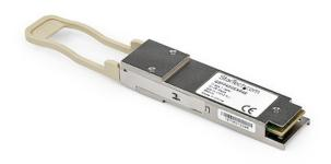
The QSFP-40G-SR4-S-ST is a Cisco QSFP-40G-SR4-S compatible fiber transceiver module that has been designed, programmed and tested to work with Cisco brand switches and routers. It delivers dependable 40 GbE connectivity over fiber cable, for 40GBase-SR4 compliant networks, with a maximum distance of up to 100 m (328 ft).
